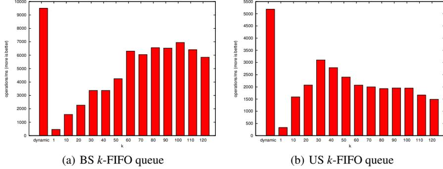
**Fig. 4.** Variable-load producer-consumer microbenchmarks with an increasing number of static  $k$  versus a dynamically controlled  $k$  on a 40-core (2 hyperthreads per core) server
